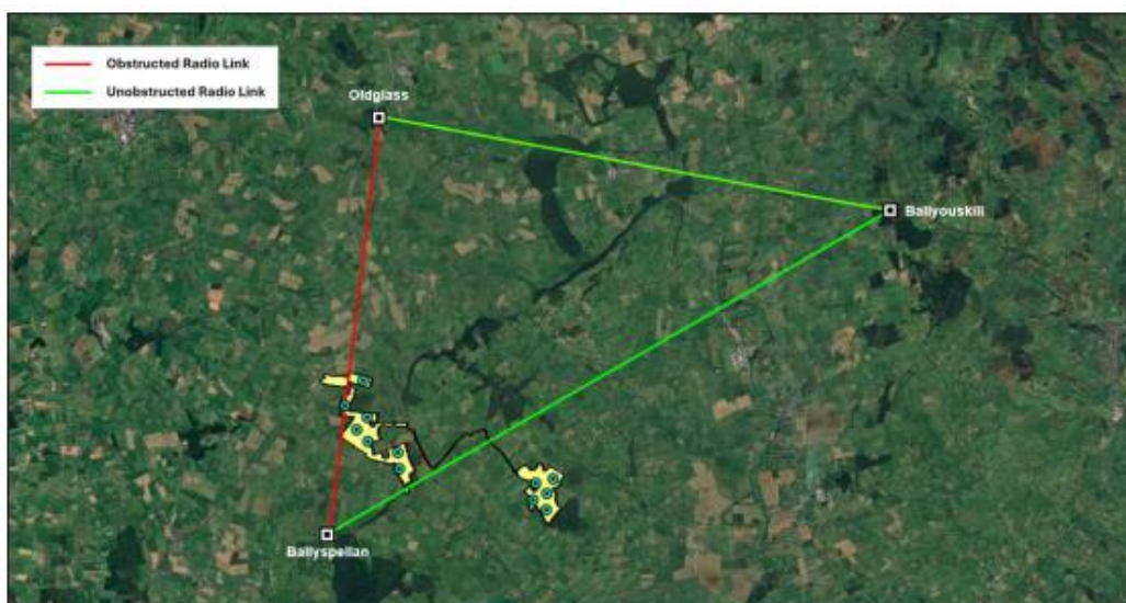
Figure 16. Example of how an existing telecoms mast could be used relay the radio link between Oldglass and Ballyspellan.
